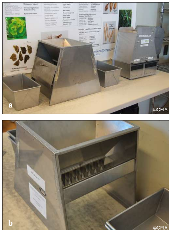
Figure 7.2. Soil (riffle) dividers: a non-tipping type (left) and tipping type (right); b detail of non-tipping type riffle divider (images courtesy of ISTA accredited laboratory CA08)
